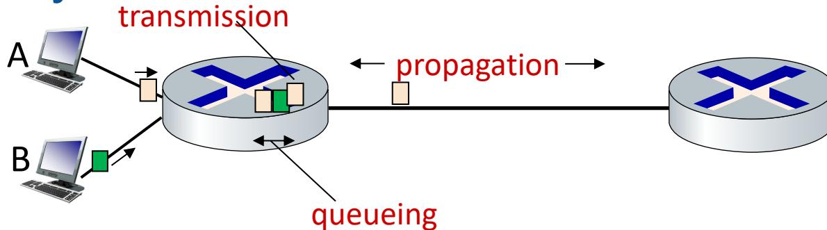
$$t_{\text{total}} = t_q + t_{\text{tx}} + t_{\text{prop}}$$
