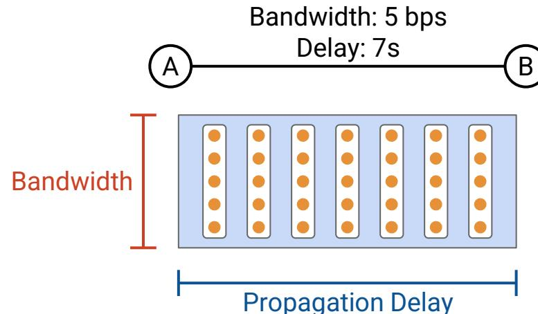
The **width of the packet** in the pipe represents the transmission delay.
