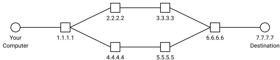
Assuming no errors occur, and our probes hit every router, then calling `traceroute` with `ip=7.7.7.7` should return something like this:
