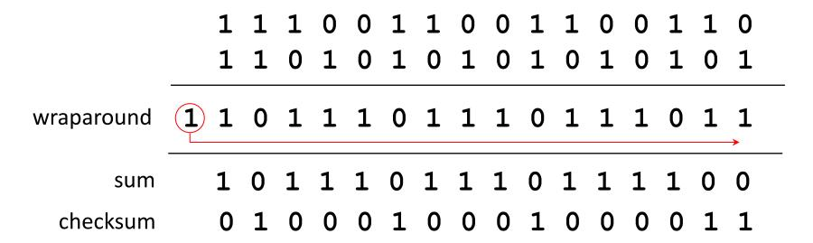
Note: when adding numbers, a carryout from the most significant bit needs to be added to the result
